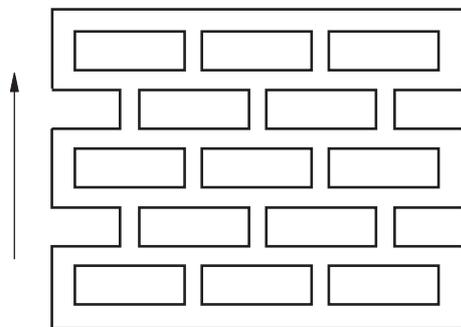
**Figure B.26 — Lightweight concrete masonry units — Geometry 1,7/1,2**
