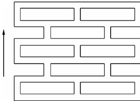
**Figure B.27 — Lightweight concrete masonry units — Geometry 1,7/0,8**
