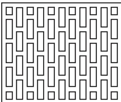
**Figure B.6 — Vertically perforated clay masonry — Geometry 1,6/3,7**
