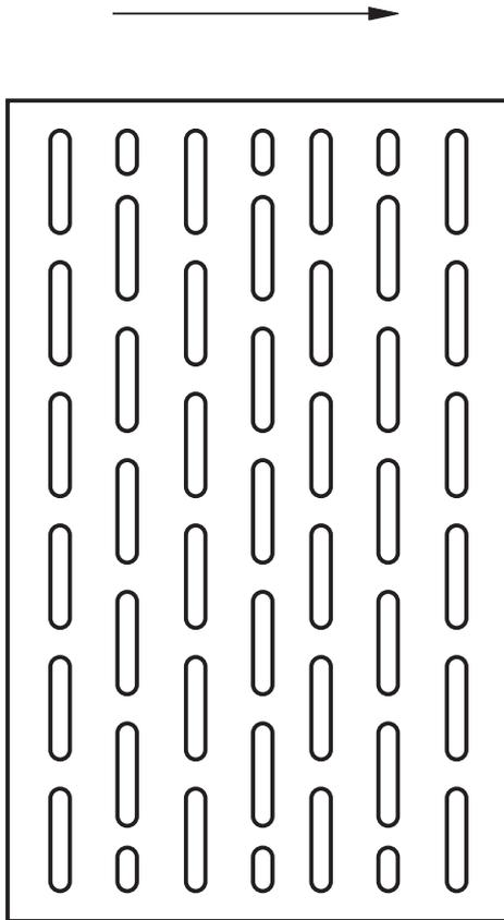
**Table B.36 — Lightweight concrete masonry units — Geometry 3,0/x**
