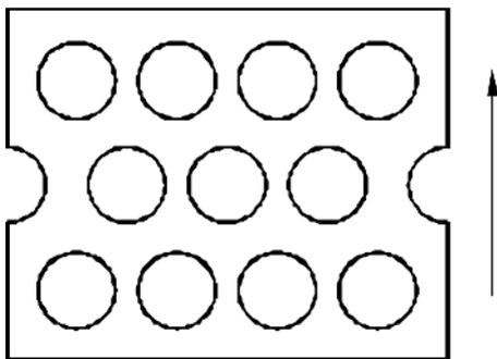
**Figure B.18 — Calcium silicate masonry units — Geometry 1,3/1,3**
