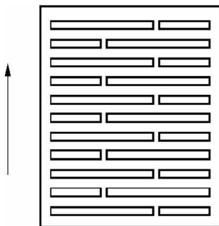
**Table B.16 — Calcium silicate masonry units — Geometry 3,7/0,8**
