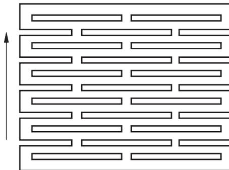
**Figure B.30 — Lightweight concrete masonry units — Geometry 3,7/0,8**
