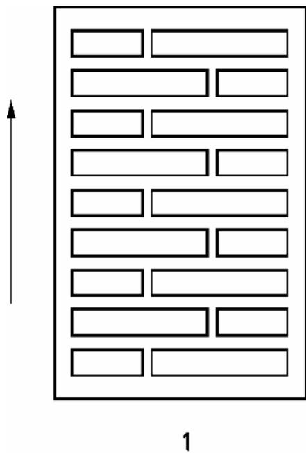
**Table B.15 — Calcium silicate masonry units — Geometry 2,5/0,8**
