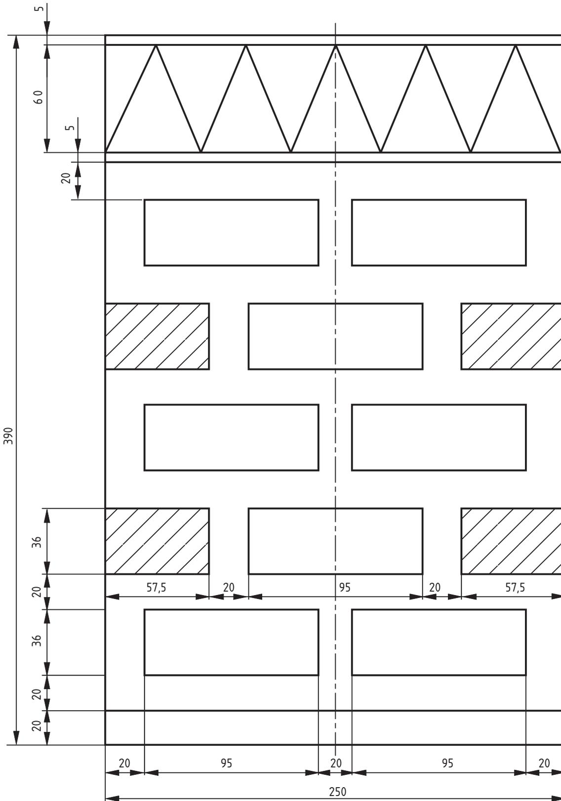
Figure D.4 — Geometry of cement bound unit
