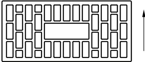
**Figure B.8 — Vertically perforated clay masonry units — Geometry 2,17/4,51**
