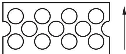
**Figure B.23 — Calcium silicate masonry units — Geometry 2,6/1,7**
