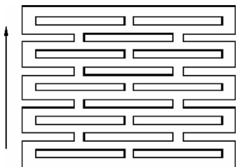
Figure B.29 — Lightweight concrete masonry unit — Geometry 3/0,8
