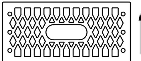
**Table B.9 — Vertically perforated clay masonry units — Geometry 3,62/3,82**
