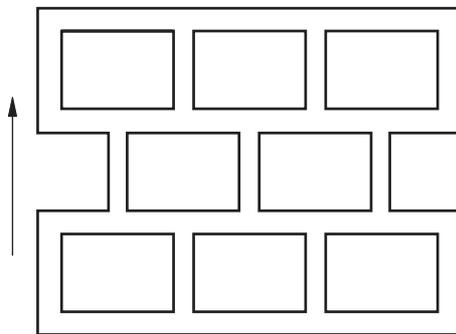
**Figure B.25 — Lightweight concrete masonry units — Geometry 1/1,2**
