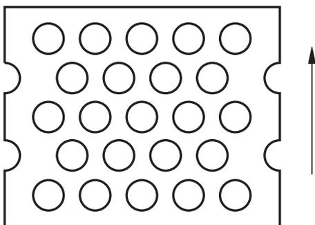
**Figure B.22 — Calcium silicate masonry units — Geometry 2,1/1,7**
