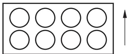
**Figure B.20 — Calcium silicate masonry units — Geometry 1,7/1,7**
