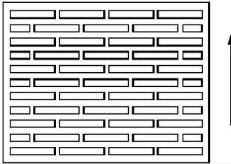
**Figure B.17 — Calcium silicate masonry units — Geometry 3,7/1,1**
