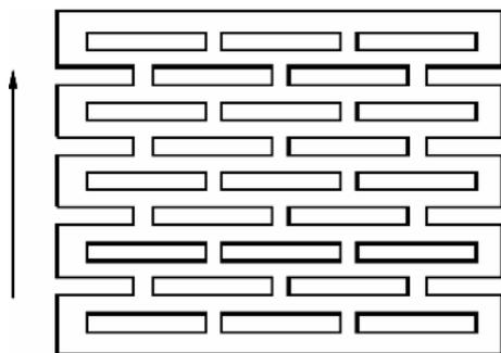
Figure B.28 — Lightweight concrete masonry units — Geometry 3/1,2
