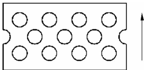
**Figure B.19 — Calcium silicate masonry units — Geometry 1,7/1,3**
